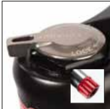
LO-R Speed Lock out Rebound adjust
