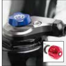
RLRC-PCS Rebound adjust Low speed Compression adjust (with PCS) Remote Lock out
